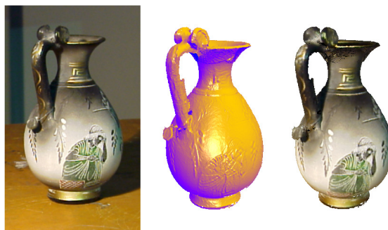
Figure 1: Left: a picture of the Greek vase model. Middle: a model reconstructed from several range images. Right: a synthetic view generated from the surface light field captured with our method. All acquired range images and pictures are registered in a fully automatic manner.
